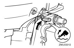
Slightly tilt the outboard motor up. The tilt support bar will lock automatically, supporting the outboard motor in a partially raised position. This outboard motor has 2 positions for shallow water cruising.
